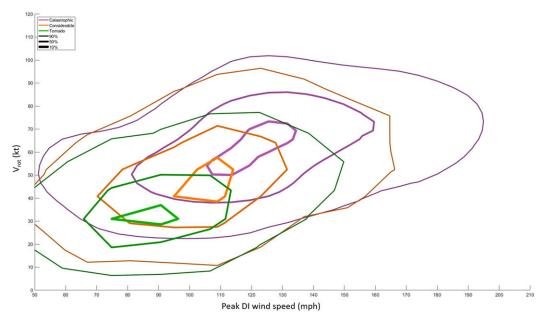
FIG. 6. As in Fig. 3, but for base-tier tornado warning (green), considerable warning tag (orange), and catastrophic tornado warning tag (purple;  $1 \text{ mph} = 0.447 \text{ m s}^{-1}$ ,  $1 \text{ kt} = 0.514 \text{ m s}^{-1}$ ).
