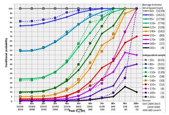
FIG. 14. Conditional probability of peak DI wind speed exceedance (legend) for an entire tornado binned for peak  $0.5^{\circ}$  scan rotational velocity (peak  $V_{\text{rot}}$ ) [kt; x coordinate, (sample size)] anywhere along a tornado path [2009–17, solid line; 2019–20, dotted line; from  $\leq 10\,000\,\text{ft}$  (3048 m) above radar level (ARL); 1 mph =  $0.447\,\text{m s}^{-1}$ , 1 kt =  $0.514\,\text{m s}^{-1}$ ].
