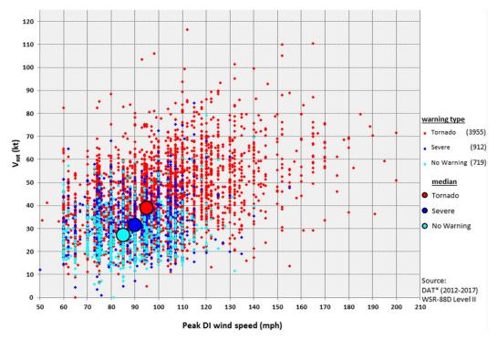
FIG. 2. Scatterplot of  $0.5^{\circ}$  DI scans by warning type (no warning, cyan; severe thunderstorm, blue; tornado, red) of peak DI wind speed (mph; x coordinate) vs  $V_{\text{rot}}$  (kt; y coordinate) during the IBW era. The large circles represent the median values of DI wind speed and  $V_{\text{rot}}$  for each warning type (1 mph =  $0.447 \text{ m s}^{-1}$ , 1 kt =  $0.514 \text{ m s}^{-1}$ ).
