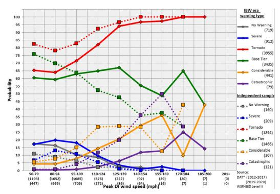
FIG. 1. Probability of impact-based warning (IBW) type vs binned wind speeds of peak damage indicators (mph; x coordinate). No warning, severe, and tornado (base-tier tornado, considerable, catastrophic) sum to 100% probability. The 2009–17 data (solid line) vs 2019–20 independent data (dotted line; 1 mph = 0.447 m s<sup>-1</sup>).
